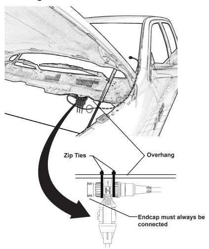
**STEP 1** - Using the supplied zip ties, fasten the EAS connectors underneath the overhang which runs across the top of the fire wall. Keep the EAS assembly close to the driver side.
